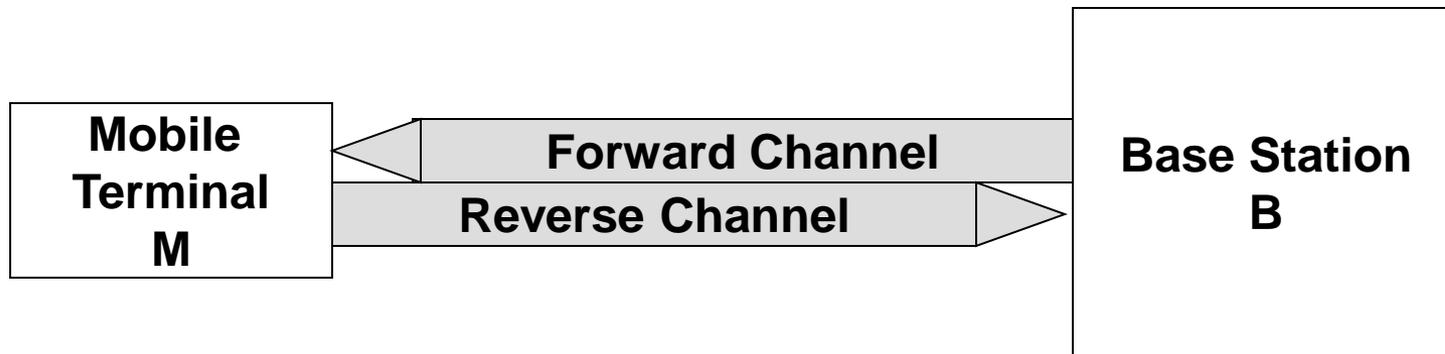
**Forward Channel and Reverse Channel use different frequency bands**
