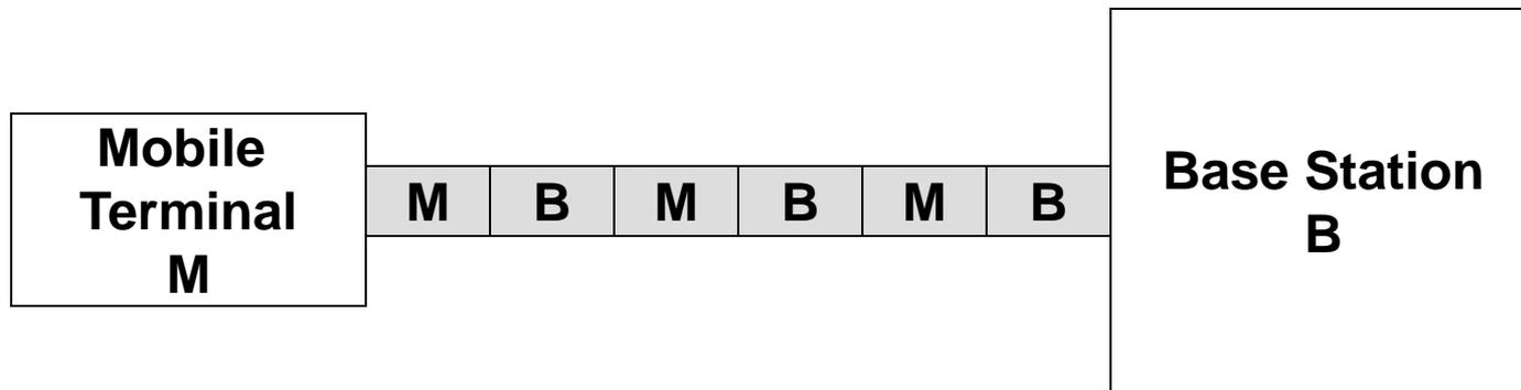
**A single frequency channel is used. The channel is divided into time slots. Mobile station and base station transmits on the time slots alternately.**
